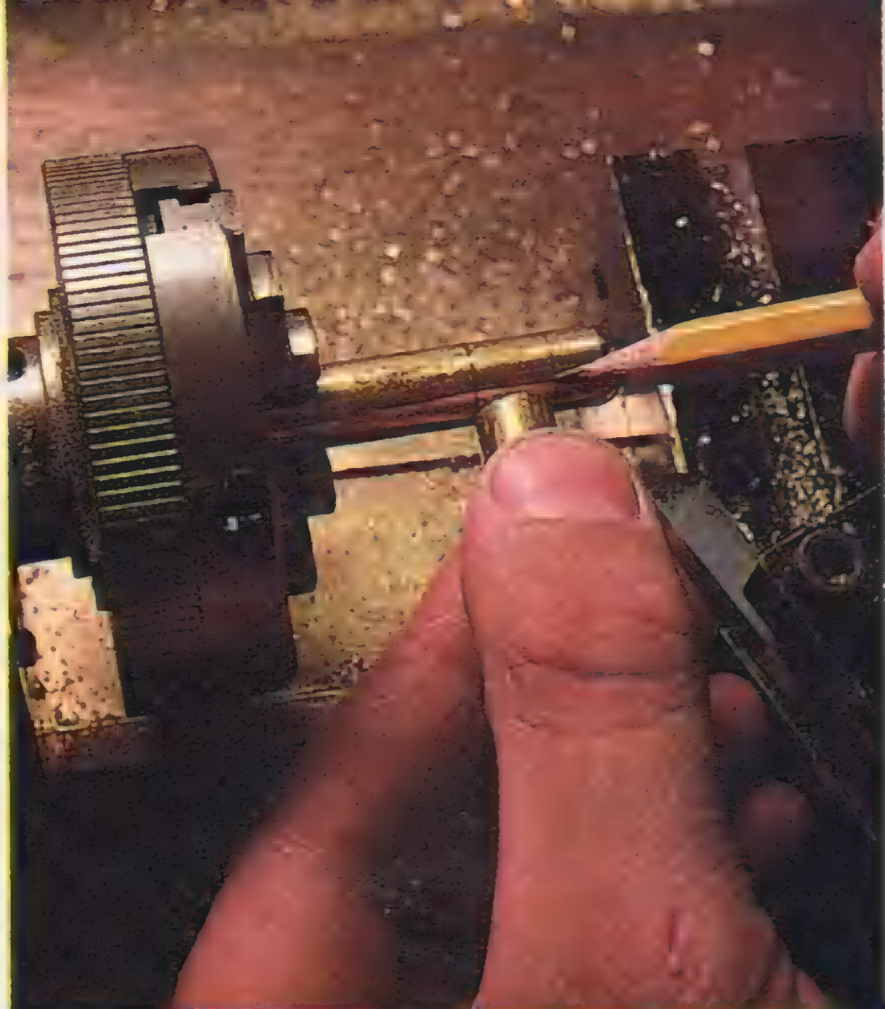
The bar stock is properly marked before turning a ball on the lathe.
